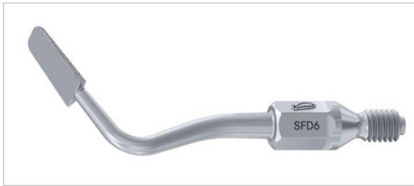
Fig 7a Special sonic tip SFD6 for the creation of a proximal (in this case, distal) preparation margin, with diamond coating on only one side to prevent trauma to adjacent teeth. The cervical edge of these sonic tips is shaped to produce the exact marginal geometry needed for high-strength dental ceramics. (Photo reproduced with permission of Komet Dental.)
